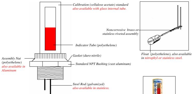
This "highly visible" gauge is recommended for use when mounting close to a tank wall and for tanks with baffles or other obstructions. It's two piece bushing (pictured right) makes it more versatile than the At-A-Glance Gauge. Direct mechanical action, reliable construction and "high visibility" make this gauge perfect choice for tanks with depths up to 12'.
