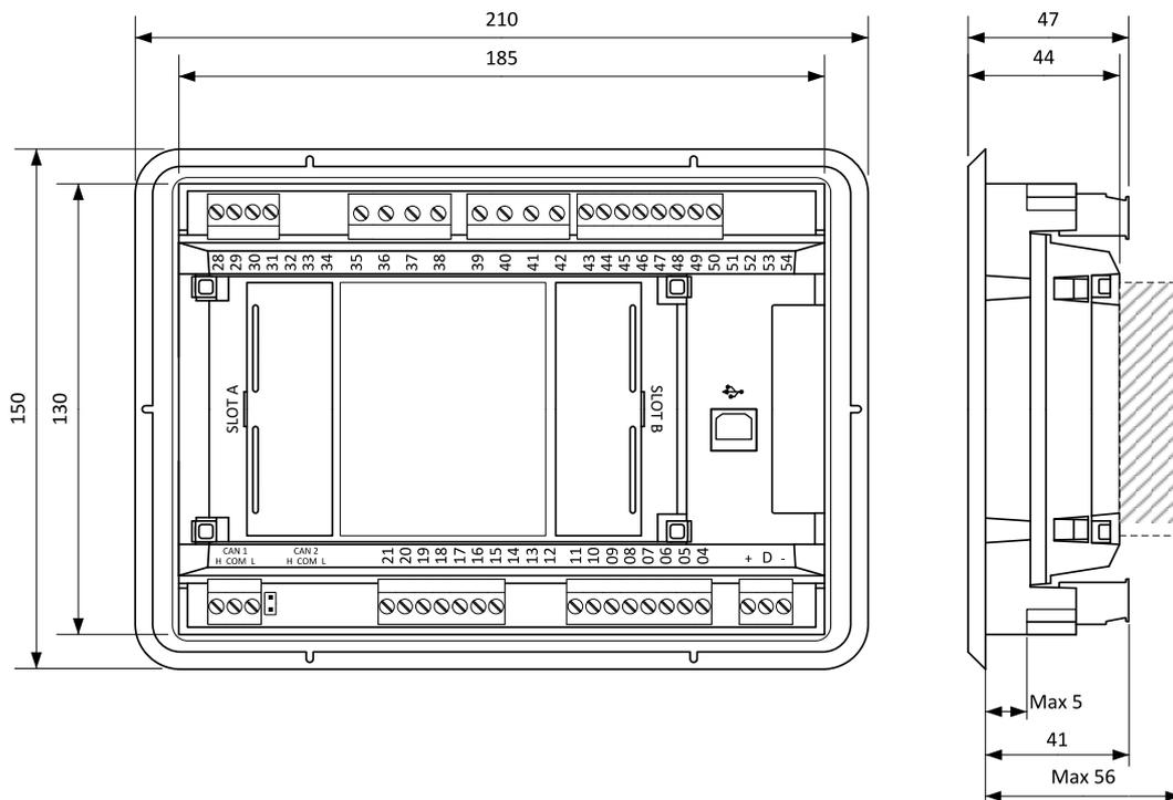
**Note:** The final depth of the controller depends on the selected plug-in module – it can vary between 41 mm and 56 mm. Mind also the size of connectors and cables (e.g. in case of RS232 connector, add about 60 mm more for standard RS232 connector and cable).
